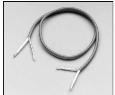
SC-182: Low inductance (42nH/ft) coaxial cable for minimizing test lead impedance in circuits using fast transient response power supplies. The cable is sold by the foot and comes without connectors. For use with: 2302, 2303, 2303B, 2303-PJ, 2304A, 2306, 2306-PJ
